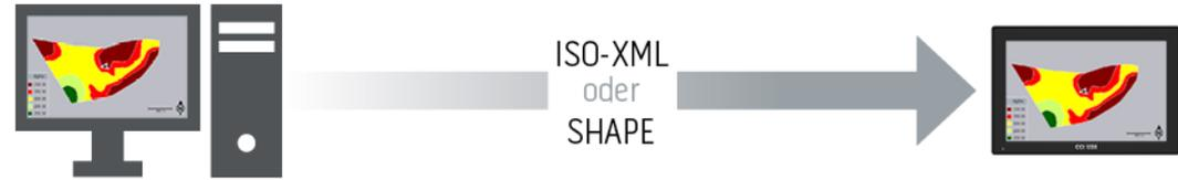
Rate Control enables the import of maps for the site-specific application in the shape or ISO-XML format.
